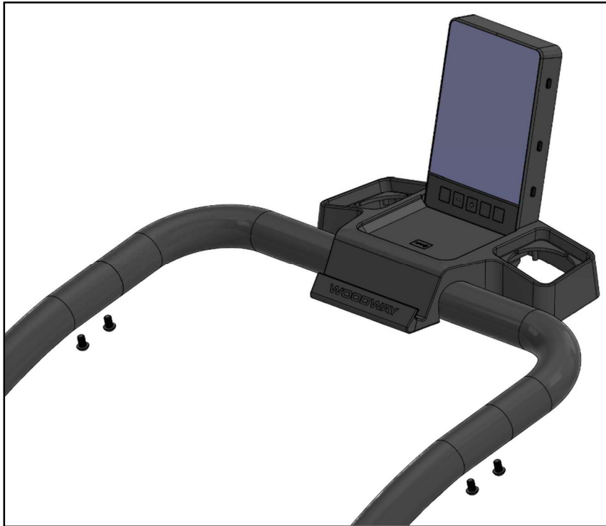
FIG. 18 Handrails and Hardware
