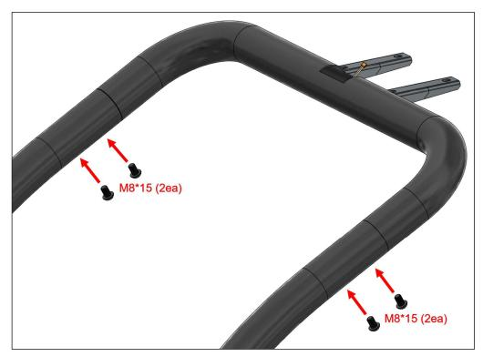
FIG. 21 Horseshoe to Handrails Hardware
