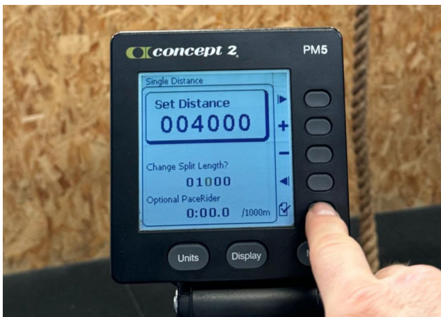
6. When 4000m set distance and split length 1000m are set press the tick button to move on
