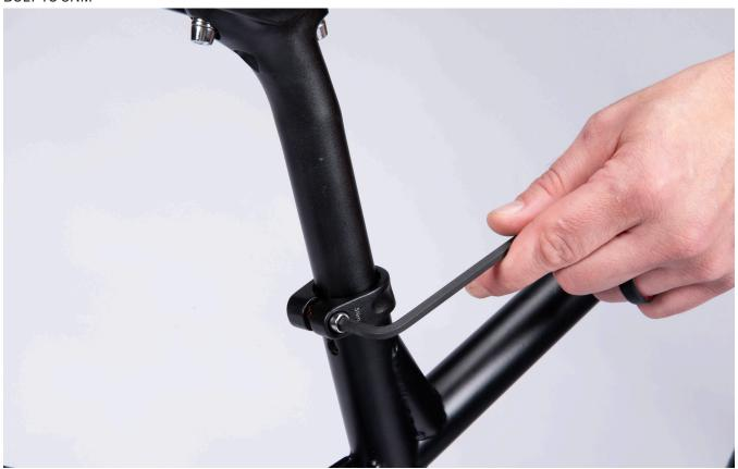
NOTE: MAKE SURE THAT THE SEAT POST DOES NOT PROJECT FROM THE FRAME BEYOND ITS "MINIMUM INSERTION" OR "MAXIMUM EXTENSION" MARK.
