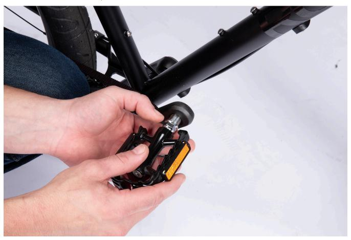
• REPEAT INSTALL WITH THE NON-DRIVE-SIDE PEDAL EXCEPT THIS WILL BE LEFT HAND THREADED. TORQUE TO 35NM WITH THE 15MM WRENCH
