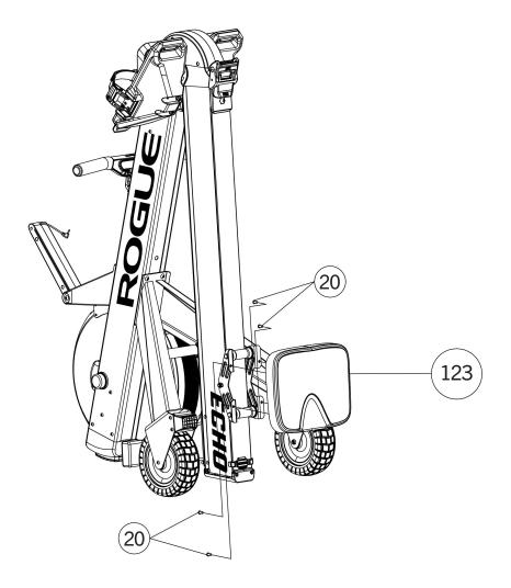
• CAREFULLY UNFOLD THE WHOLE UNIT BY PLACING A FOOT ON ONE OF THE REAR TIRES, RELEASING THE HINGE LATCH AND SLOWLY OPENING THE ROWER OUT INTO A HORIZONTAL POSITION
