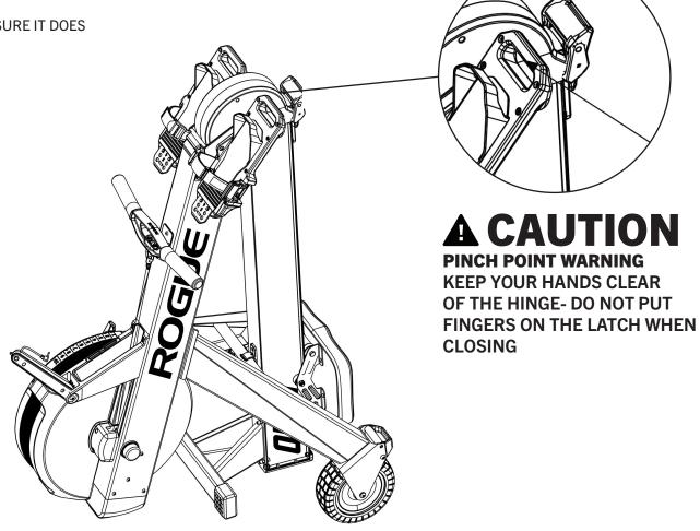
• TO SECURELY LOCK THE ROWER MAIN FRAME (80) LIFT THE LATCH HANDLE FULLY FORWARD UNTIL IT CATCHES THE HOOK THEN PULL THE HANDLE BACK DOWN AND PUSH IT FIRMLY CLOSED
