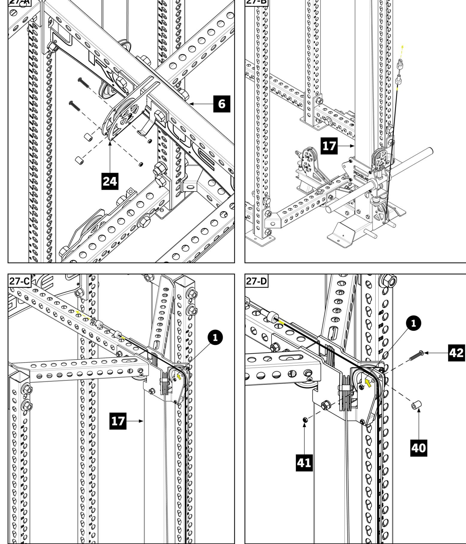
Pull cable past the Nameplate Crossmember [6]. Feed cable around the Lat Pulldown Pulley Bracket [24] shown in 28-A.
