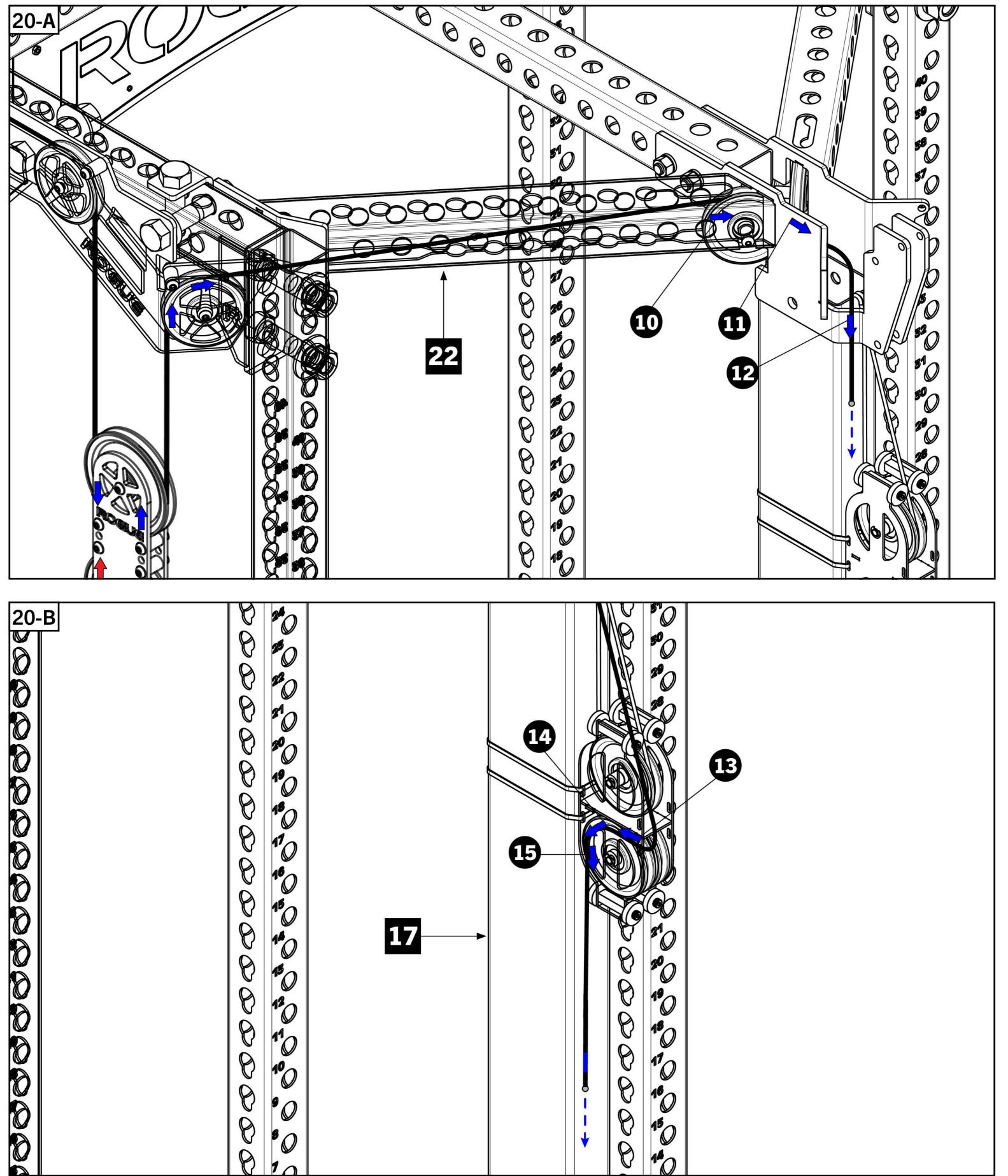
Continuing down towards the Plate Load Trolley, feed cable around the Pulley located on top of the Plate Load Trolley.
