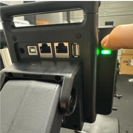
2. Press until the light turns green, indicating the monitor is in comp mode
