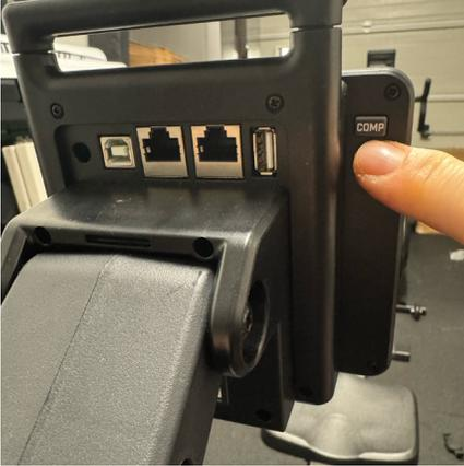
1. Press the comp mode button on the back of the monitor
