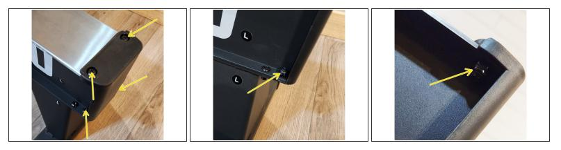
• Using the T27 wrench and the 11mm wrench, remove the 4 screws and accompanying nuts (2 on the top and 2 on the bottom) of the slide rail end cap.
