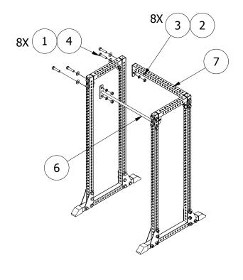
STEP 2: ATTACH PULL-UP BAR & CROSSMEMBER TO SIDE FRAMES. SECURE USING 1" x 4.75" HEX BOLTS, 1" FLAT WASHERS, 1" LOCK WASHERS, AND 1" HEX NUTS.
