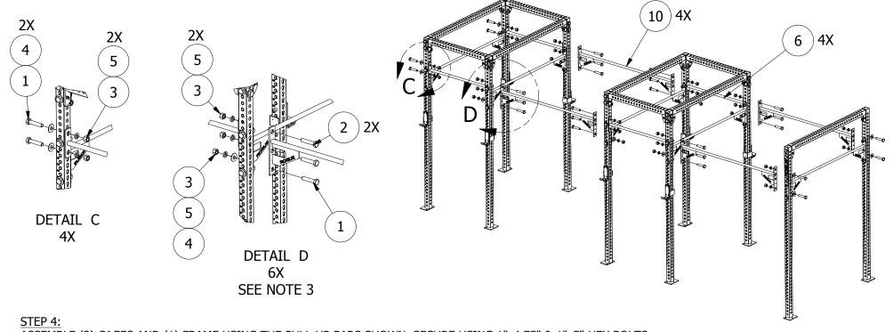
ASSEMBLE (2) CAGES AND (1) FRAME USING THE PULL-UP BARS SHOWN. SECURE USING 1"x4.75" & 1"x5" HEX BOLTS, 1" FLAT WASHERS, 1" LOCK WASHERS, 1" HEX NUTS.
